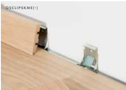
CLIPS 1 pack: 50 clips Place one clip every 0.5 m along the wall and click the skirtings to the clips. Not compatible with 12 mm floors.
